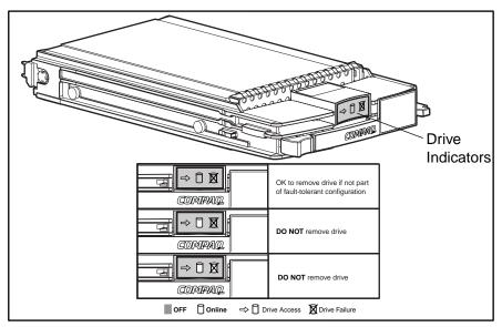
Figure 4-14. Hot-Plug hard drive LEDs and replacement conditions
